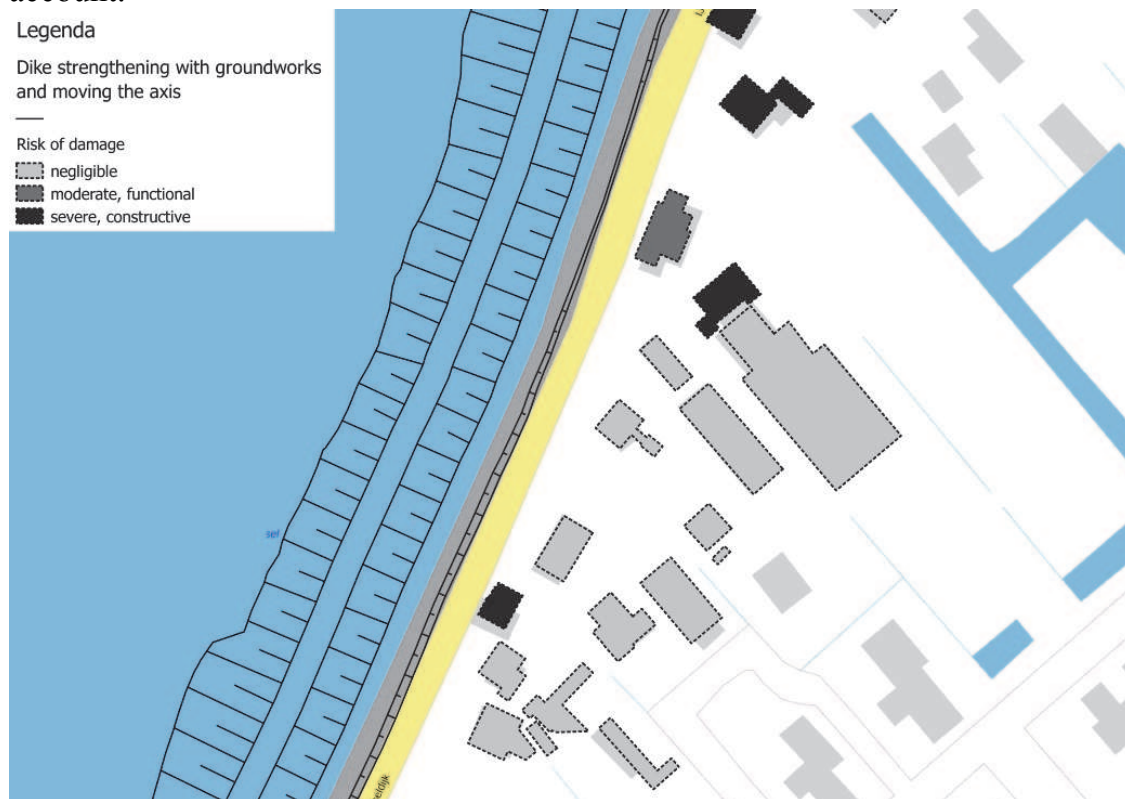
Fig.8 : Damage risk assessment for design alternative four
